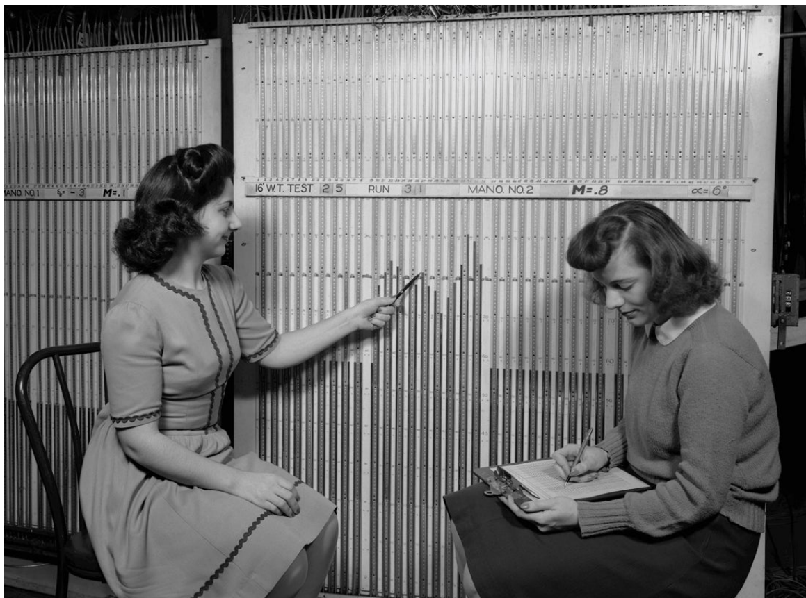
NACA Ames computers reading the manometer (pressure measurements) board for the 16 ft wind tunnel and calculating the test data 1943 photograph Collection of NASA ARC-1943-AAL-4962 R2022.2201.013
