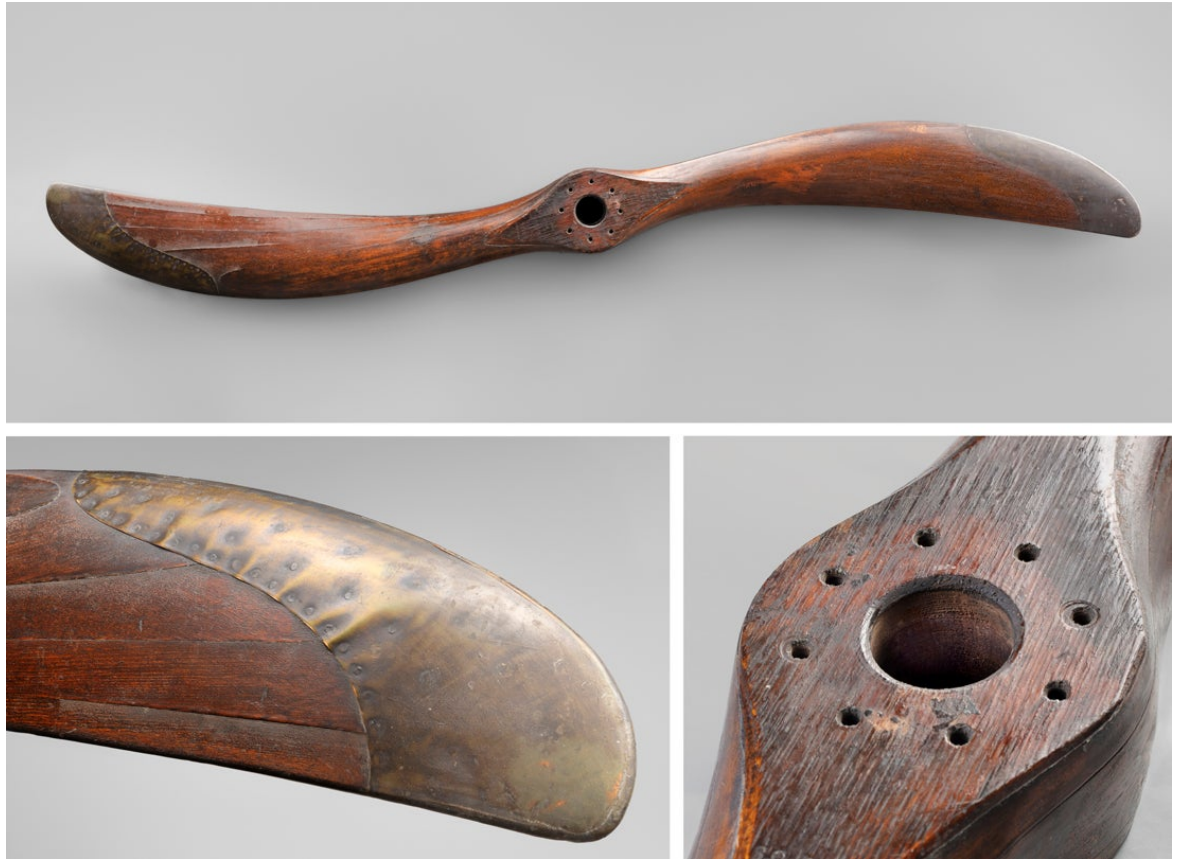
Paragon Striker propeller c. 1918 American Propeller and Manufacturing Company, Baltimore, Maryland wood, copper, steel Collection of Wings of History Air Museum, San Martin, California L2020.2403.001
