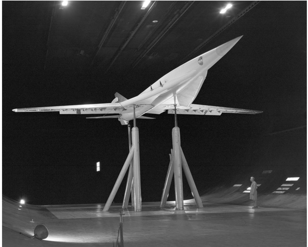
Supersonic transport configuration model in 40 x 80 wind tunnel 1964 photograph Collection of NASA A-33012 R2022.2201.006
