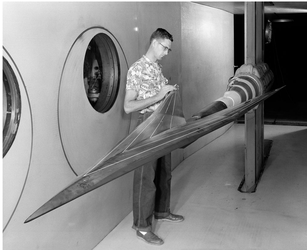
An arrow-wing model in the 6 x 6 supersonic wind tunnel 1958 photograph Collection of NASA A-24035 R2022.2201.004
