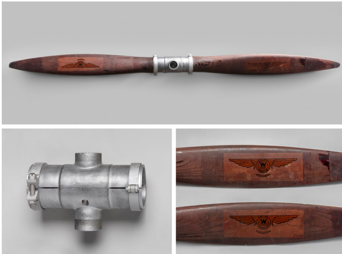
Westinghouse Micarta propeller and ground adjustable hub late 1920s Westinghouse Electric and Manufacturing Company, Pittsburgh, Pennsylvania Bakelite plastic, canvas, metal, decals Courtesy of the Monte Chase, Not Plane Jane Propeller Collection, Mandan, North Dakota L2020.2402.001
