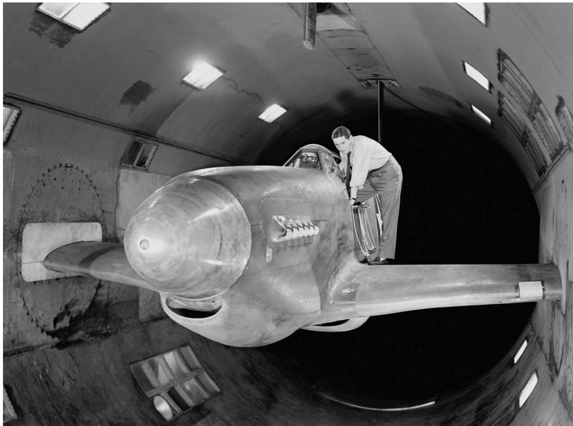
North American XP-51B Mustang airplane with outer wing structures removed in 16 ft wind tunnel 1943 photograph Collection of NASA ARC-1943-AAL-3782 R2022.2201.012
