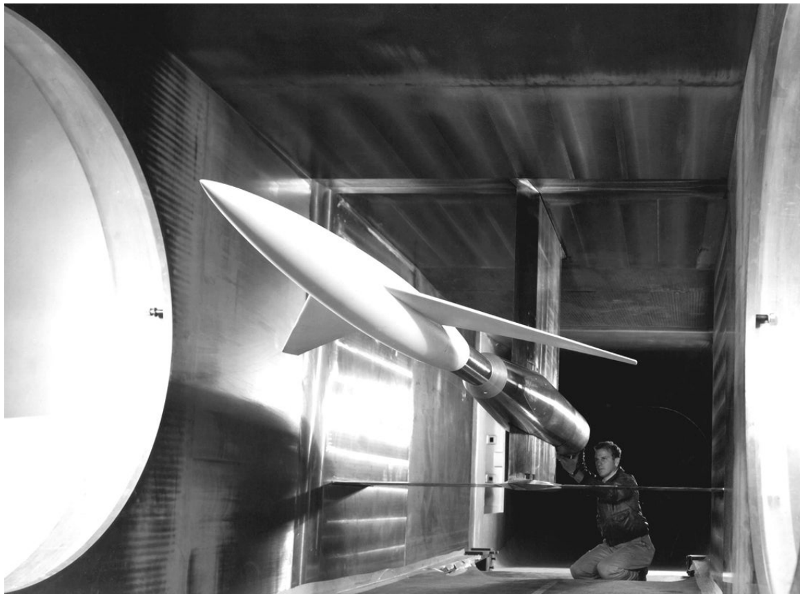
Swept-wing model mounted in the 6 x 6 supersonic wind tunnel 1948 photograph Collection of NASA A-1743 R2022.2201.001
