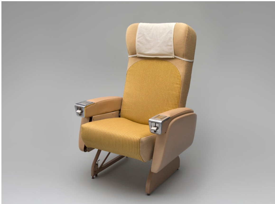
TWA (Trans World Airlines) Lockheed L-1049 Super Constellation seat 1950s TECO, Inc. metal, fabric, foam rubber Collection of SFO Museum Gift of Airline History Museum at Kansas City 2000.093.001 a L2023.0401.014
