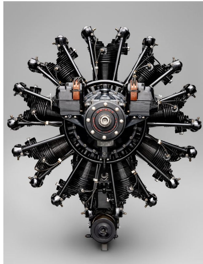
Wright J-5-A R-790 Whirlwind radial aircraft engine 1929 Manufacturer's number 13638 Wright Aeronautical Corporation, Paterson, New Jersey aluminum, steel, rubber, phenolic Courtesy of the Frederick W. Patterson III Collection L2020.2401.002
